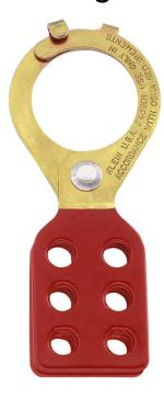
The Klein Tools Lockout with Interlocking Tabs is designed to lock out power sources, such as disconnects, switches and panel boxes. The lockout has zinc-plated double interlocking hasps of tempered steel with interlocking tabs for extra security. Tabs feature 6-hole locking bodies coated with red vinyl plastic.
